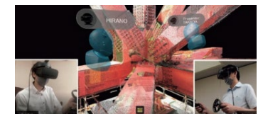
3D workability review using point cloud data
