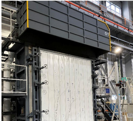
Exterior wall fireproof test (product development)
