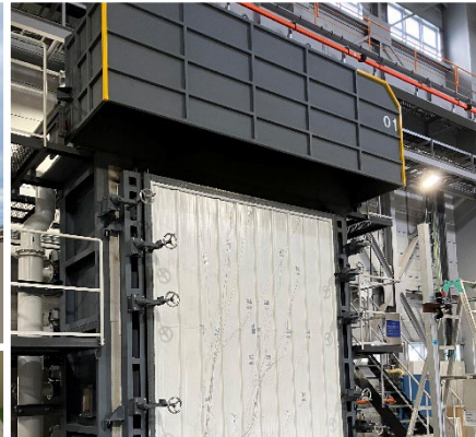
Exterior wall fireproof test (product development)
