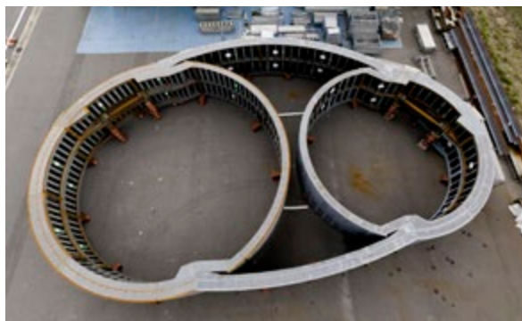
Temporary assembly of a steel tunnel segment
