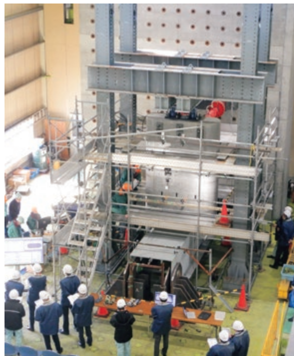
Load testing of rigid connection of superstructure and substructure for Tamagawa Sky Bridge
