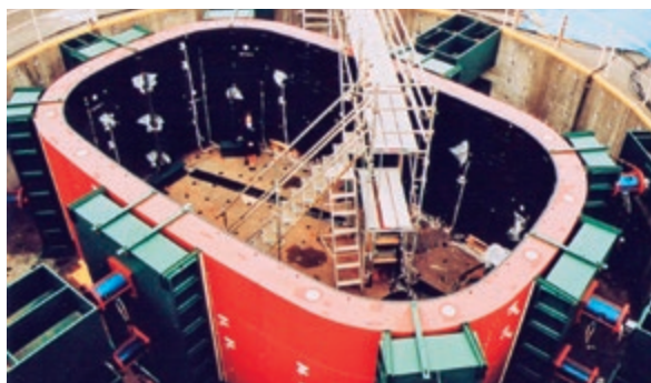
Actual-size ring loading test
