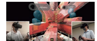
3D workability review using point cloud data
