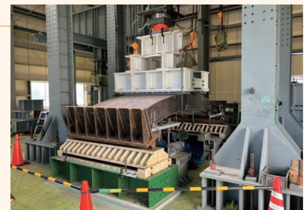
Bending performance confirmation test for five-sided steel shell composite segments
