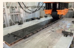
Moving wheel load test for rationalized joints
